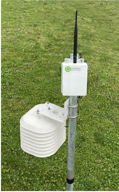
LE CAPTEUR TEMPÉRATURE ET HYGROMÉTRIE POUR L'EXTÉRIEUR COMPATIBLE RÉSEAU "INTERNET DES OBJETS" SANS WI-FI, SANS BLUETOOTH, ET SANS GSM !
